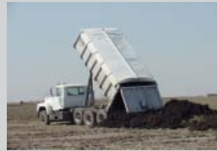
Biosolids are hauled in trucks with sealed end gates and covered boxes.
