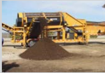
Yard and garden compost is screened to remove debris prior to mixing with biosolids.
